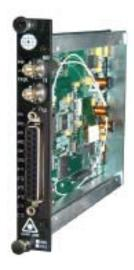
Digitally Encoded Two Bi-directional Contact Closure and Two Full Duplex RS-422 Data (Manchester, Bi-Phase)
