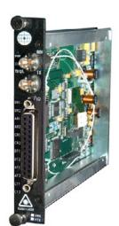
Digitally Encoded Two Bi-directional Contact Closure and Two Full Duplex RS-422 Data (Manchester, Bi-Phase)
