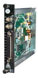
Digitally Encoded One Bi-directional 24-bit Audio and Two Full Duplex RS-422 Data (Manchester, Bi-Phase)
