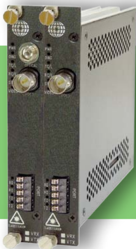
FXA/FXB-1HG2A/1HG2A-x 3G-SDI Video and BALANCED AUDIO w/ Screw Terminal connector
