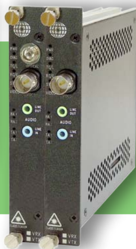
FXA/FXB-1HG2AB/1HG2AB-x 3G-SDI Video and UNBALANCED AUDIO w/ 3.5mm Stereo connector
