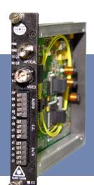
Digitaly Encoded One 10-Bit 10MHz Video Mux with Two Bi-directional Contact Closure, One Full Duplex Multiprotocol Data and One Return Channel of Extended Range Pelco or Panasonic "up-the-coax" Control Data
