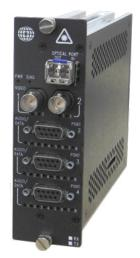
Digitally-Encoded Two Channels 8-bit Video with Two Bi-directional 24-bit Unbalanced Audio and Eight Bi-directional RS-232 Data using the Industry Standard Small Form Pluggable (SFP) Optical Device
