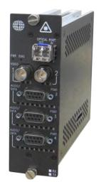
Digitally-Encoded Two Channels 8-bit Video with Two Bi-directional 24-bit Audio and Eight Bi-directional RS-232 Data using the Industry Standard Small Form Pluggable (SFP) Optical Device
