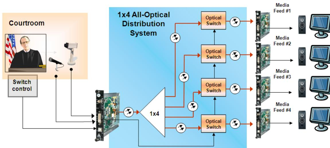
All-optical routing and switching adds capabilities to the transport and routing system not presently available in copper-based systems. By keeping the signals in the optical domain, the quality of the signals (video & audio) is maintained since conversion to and from the electrical domain is done primarily at the end points of the system.
