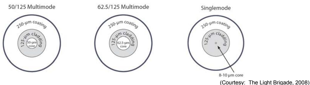
The basic rule of thumb is that the smaller the core diameter, the higher the fiber's bandwidth and the lower the attenuation (loss in dB per kilometer). The fiber's attenuation and bandwidth are also dependent on wavelength. The table below illustrates the approximate attenuation of both multimode & singlemode fibers.
